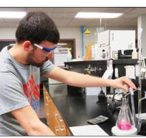
Water Operations intern Aaron Jewell tests titrations which determines end-point of water samples.
