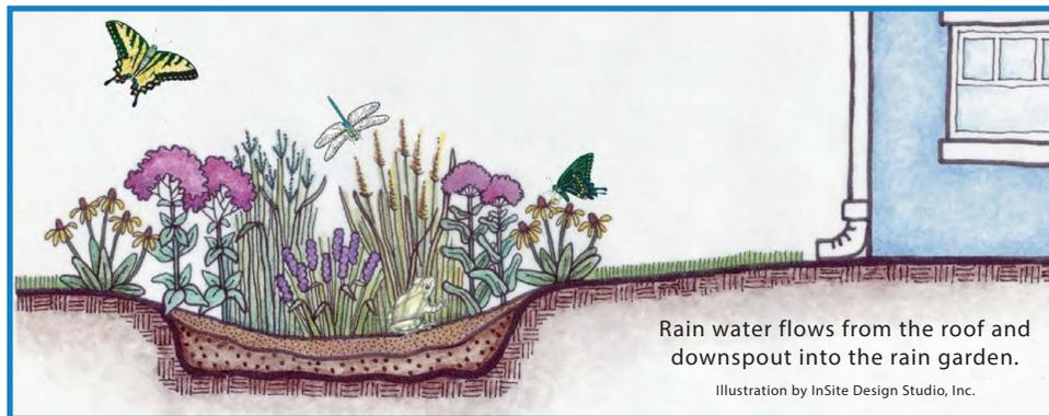
Rain water flows from the roof and downspout into the rain garden.
